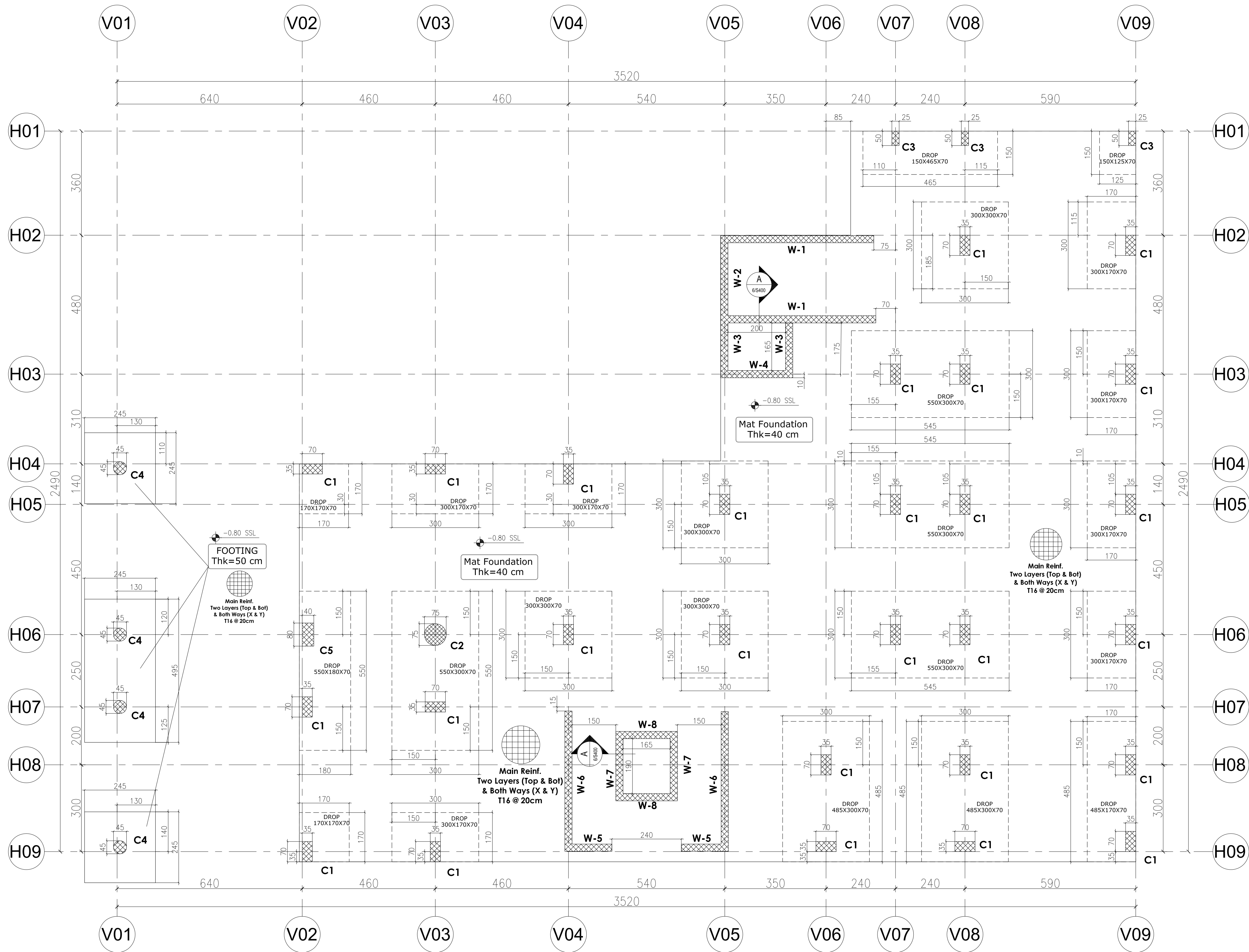
1 MAT FOUNDATION GENERAL ARRANGEMENT PLAN S-500 SCALE 1:75
